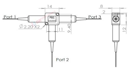
1. Optical Path: Port 1 Input, Port 2 /Port 3 output, Port 3 Panda fiber is aligned to P1.
