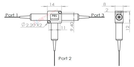
1. Optical Path: Port 1 Input, Port 2 /Port 3 output, Port 3 Panda fiber is aligned to P1.
