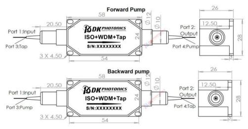
$\star$  For forward pump, Tap is both axis working. For backward pump, Tap is fast axis blocked, slow axis working. Both types pump is both axis working.
