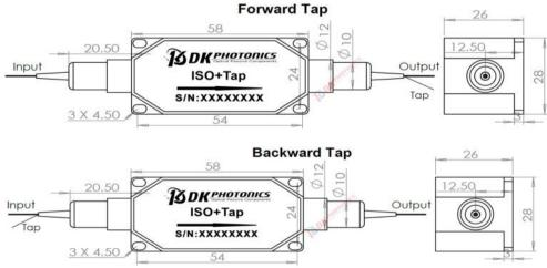
\* If Tap port is on the input side (Backward Tap), Tap is both axis working. If Tap port is on the Output side (Forward Tap), it is fast axis blocked, slow axis working. The default tap is on the input side.
