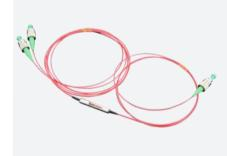
The Polarization Maintaining Tap Coupler is a polarization maintaining coupler which splits the light from the input PM fiber into two output PM fibers. The state of polarization can be aligned either with the slow axis or the fast axis of the PM fibers. The rugged stainless-steel package is designed for high optical performance and stability. This compact device offers low excess insertion loss, low back reflection, and high extinction ratio. Split ratios from 1% to 50% are available.
